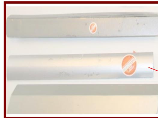
Cash traps are simple pieces of plastic trunking sprayed to match the colour of the machine and placed across the cash slot to stop cash coming out.
